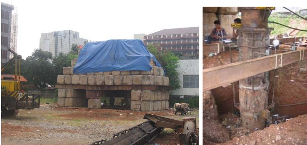
**Figure 3. Loading test on progress (left) Cracks on pile during loading test (right)**
