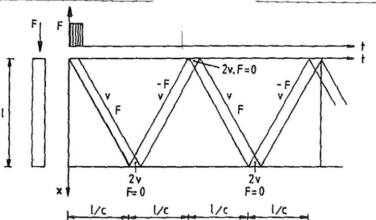
Fig. 6 : Response of a free ended prismatic bar on a pulse load at the top
