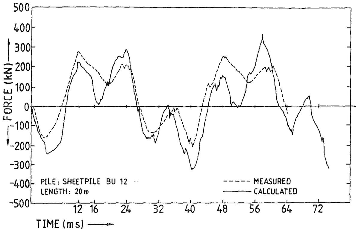
Fig. 13 : Comparison Measured and Calculated Force-time diagrammes
