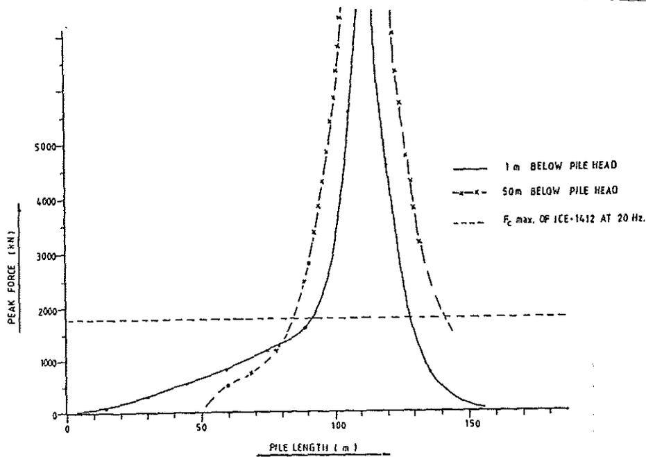
Fig. 11 : Max. Peakforce vs Pile length
