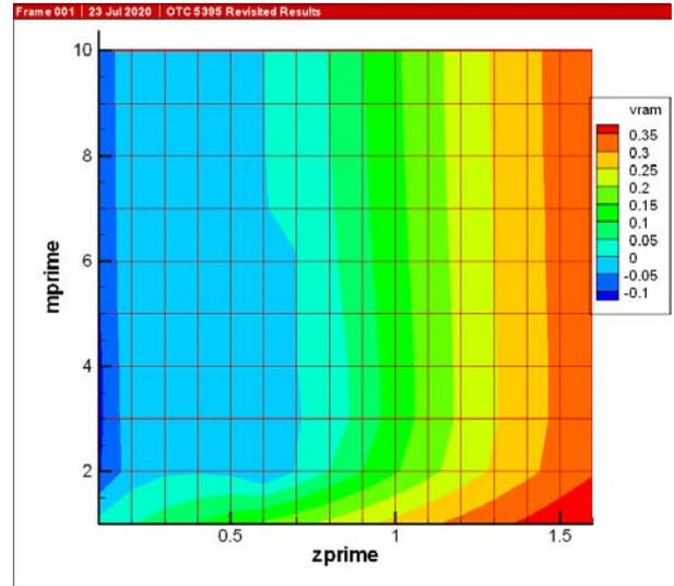
Figure 4. Ram Velocity after Impact, Parametric Study
