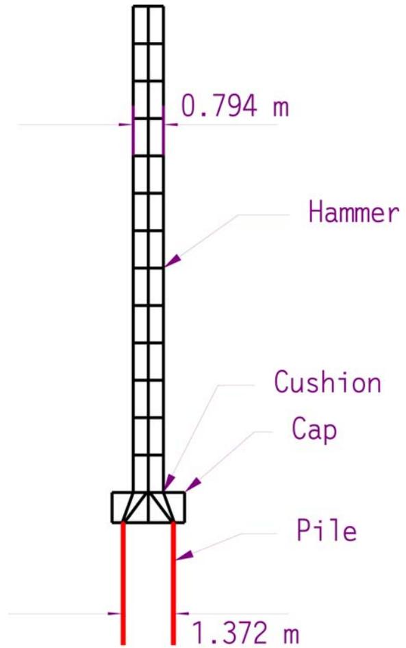
Figure 18. STADYN Axisymmetric Model for Ram, Cap and Pile Top
