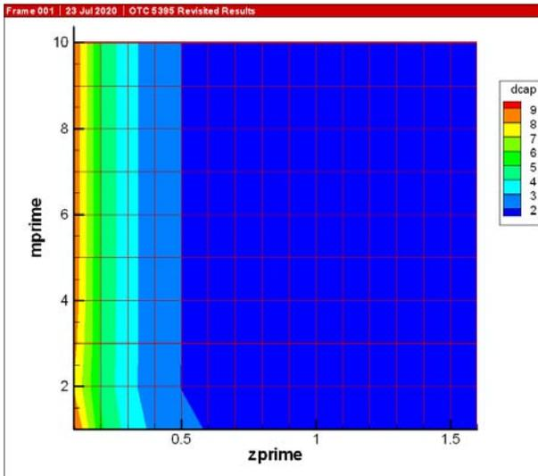
Figure 10. Maximum Pile Head Displacement, Parametric Study
