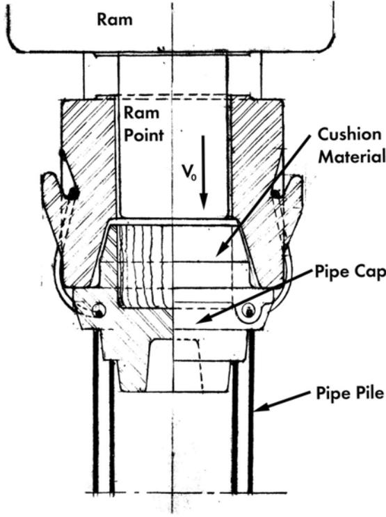
Figure 1. Hammer-Cap-Pile System
