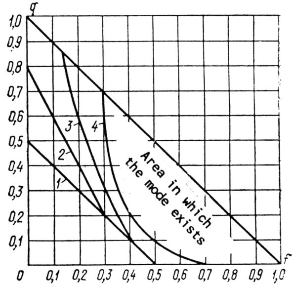
Figure 12. Area in which the mode of pile displacement being studied exists 1:  $\gamma = 1.6$ ; 2:  $\gamma = 1.3$ ; 3:  $\gamma = 1.0$ ; 4:  $\gamma = 0.7$  (modified from Tseitlin et al. (1987))
