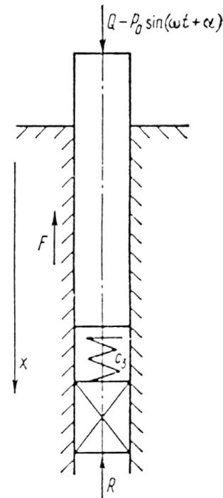
Figure 17. Vibratory model with toe elasticity (from Tseitlin et al. (1987))
