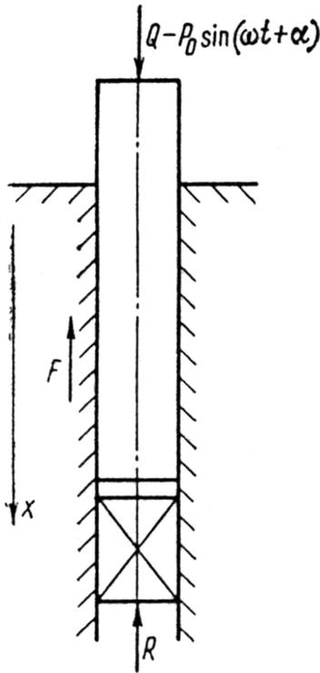
Figure 3. Computational diagram for vibrational driving using longitudinal vibrations (from Tseitlin et al. (1987))
