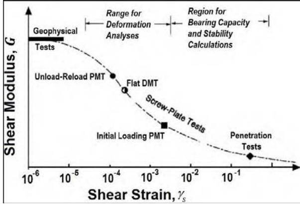
Figure 5. Typical Values of Shear Modulus Based on Field Tests (from Loehr, Lutenegeger, Rosenblad, and Boeckmann (2016))
