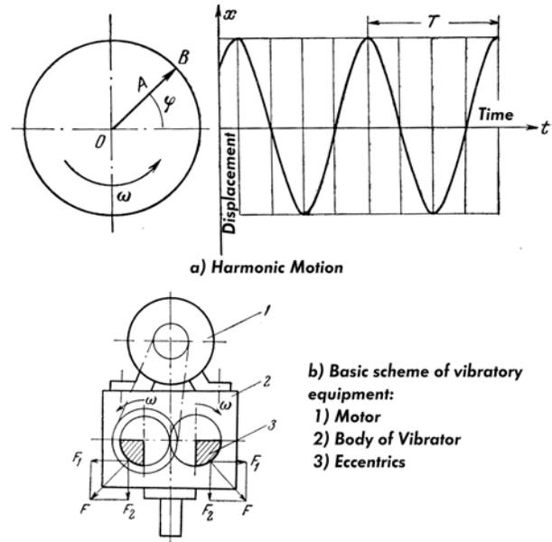
Figure 2. Basics of Vibratory Technology and Pile Drivers (modified from Rebrik (1966))
