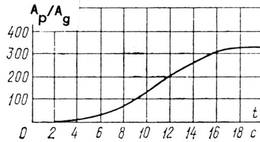
Figure 4. Amplitude Ratio vs. Time Between Pile and Ground (from Tseitlin et al. (1987))
