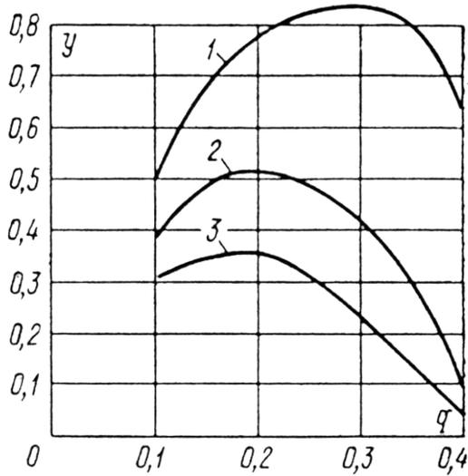
Figure 7. Dimensionless displacement  $y$  as a function of parameter  $q$  with  $f = 0.5$  and 1:  $\gamma = 0.7$ ; 2:  $\gamma = 1.0$ ; 3:  $\gamma = 1.3$  (from Tseitlin et al. (1987))
